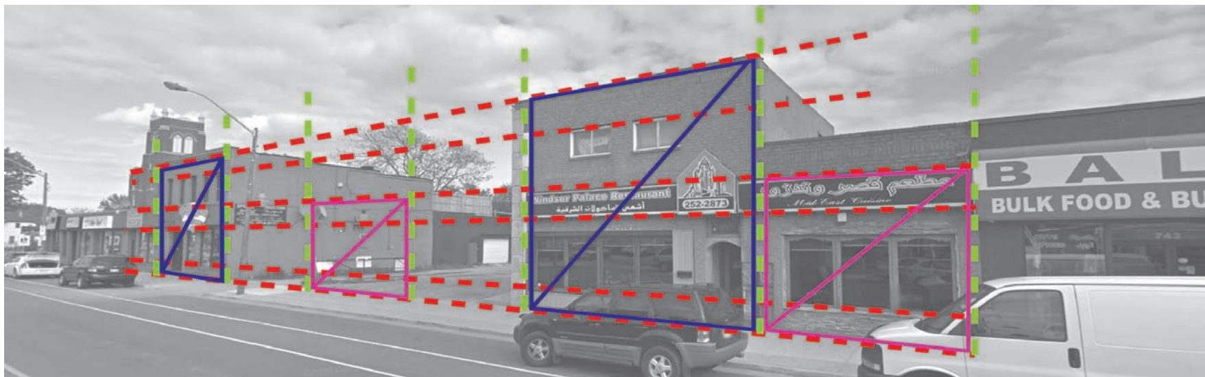
Figure 82. Regulating lines and building proportions identify a pattern along the Wyandotte Towne Centre BIA Mainstreet on the south side from Louis to Marentette Avenue that can be used for infill development.
