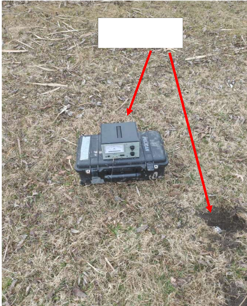
D1: Accelerometer and Ground Mounting Spike
