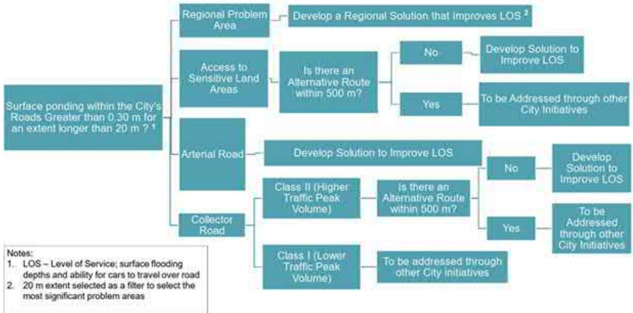
**Figure 6-5: Flow Chart – Decision-Making Process - Surface Flooding Solutions**
