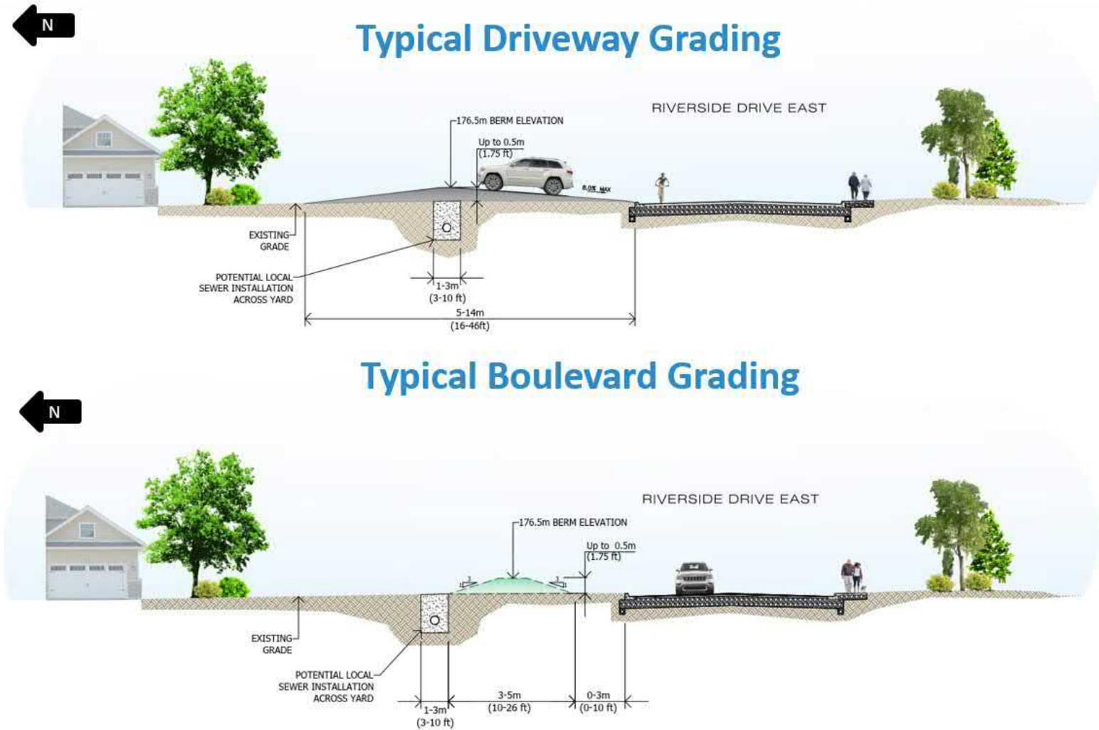
Figure 6-41: Typical Cross Section for the Alternative 1 Landform Barrier in Area 1 (BERM-E1)
