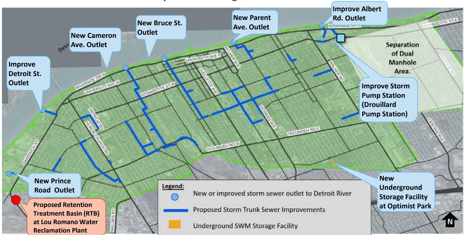
These improvements include the construction of 4 new storm sewer outlets and improvement to 2 existing outlets. This solution requires the direction of both municipal and private property drainage, such as drainage from roofs, front and rear yards and alleys, to the storm sewer system and out of the combined sewage system.
