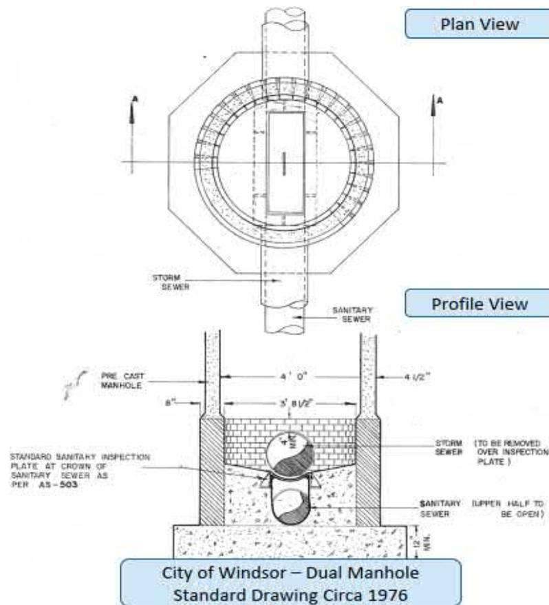
**Figure 5-5: Dual Manhole Standard Drawing**
