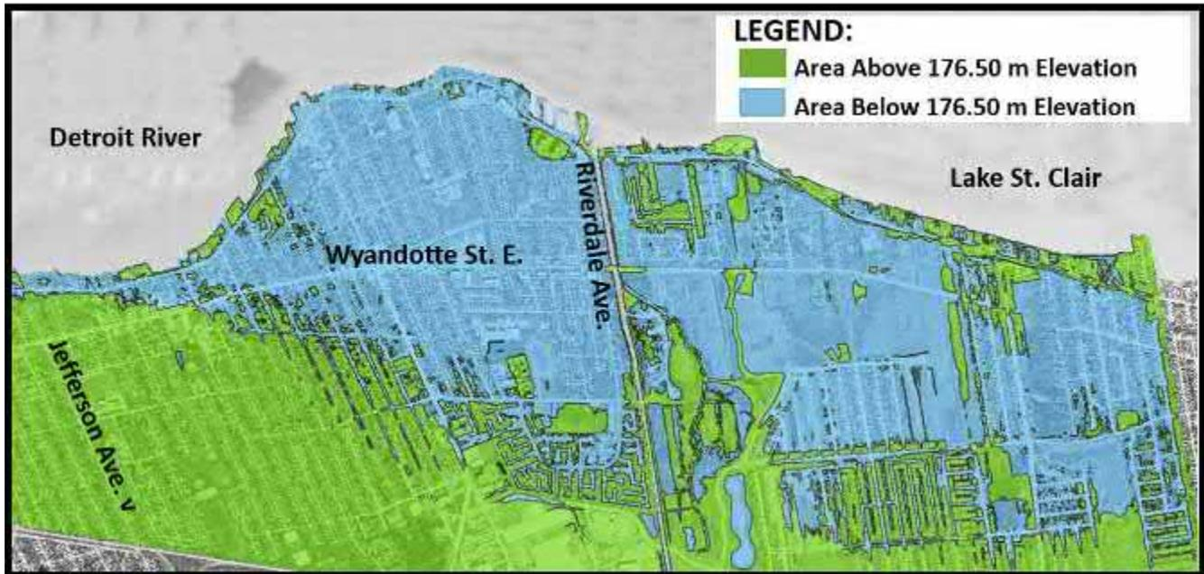
The recommended landform barrier will be an earth berm built to an elevation of **176.50**, located along the North or South boulevard of Riverside Drive East. Construction of the berm will require:
