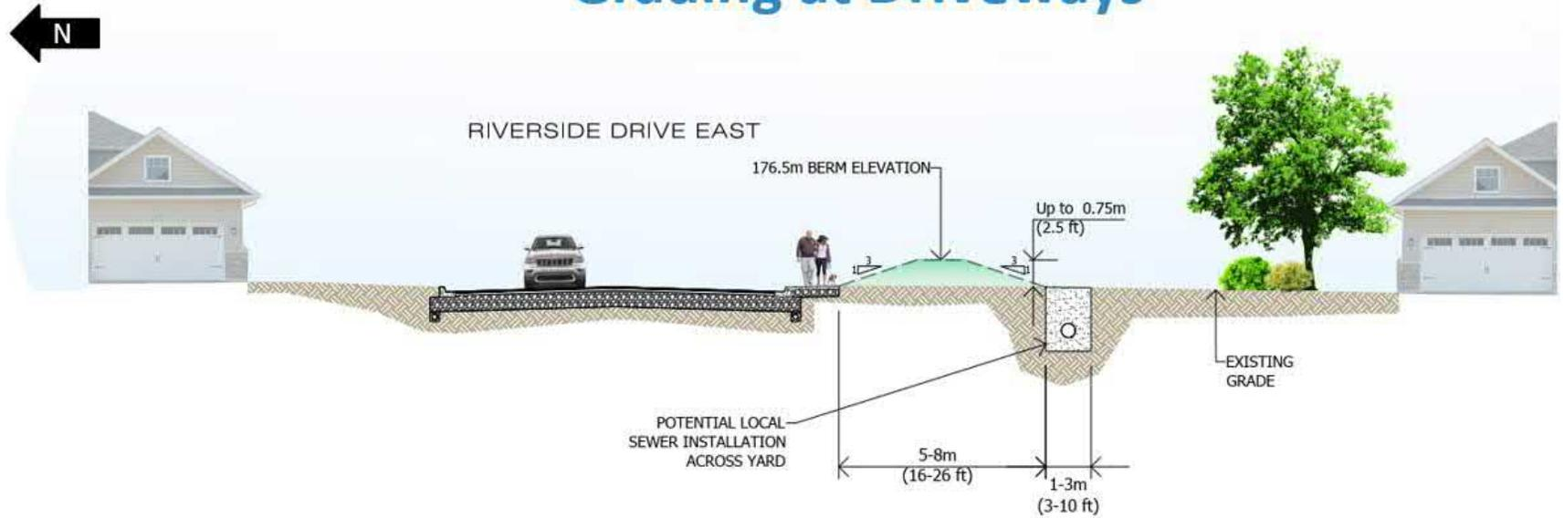
Figure 6-42: Typical Cross Section for the Alternative 1 Landform Barrier in Area 2 (BERM-2)
