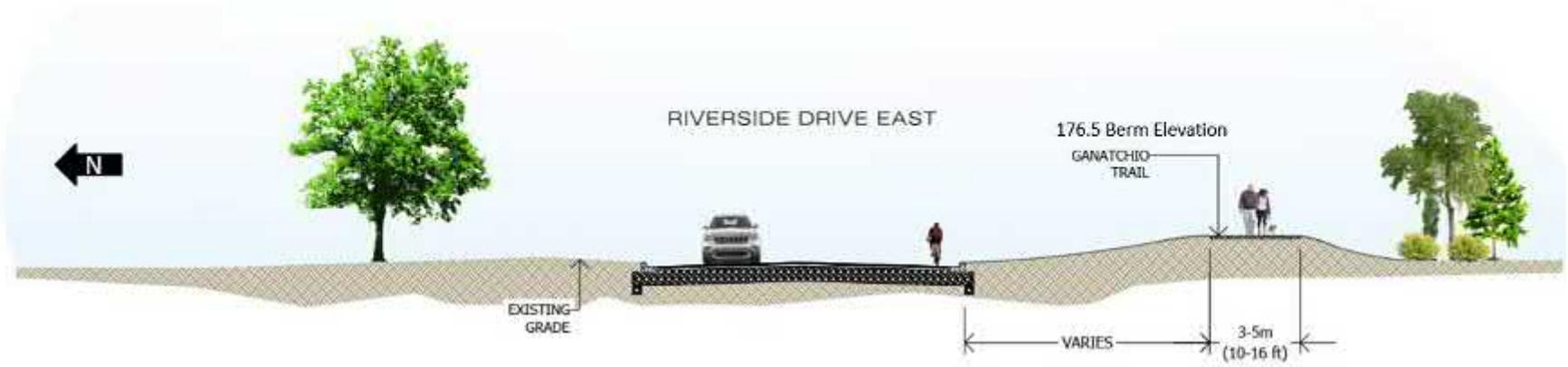
Figure 6-43: Typical Cross Section for the Alternative 1 Landform Barrier in Area 1 (BERM-3)
