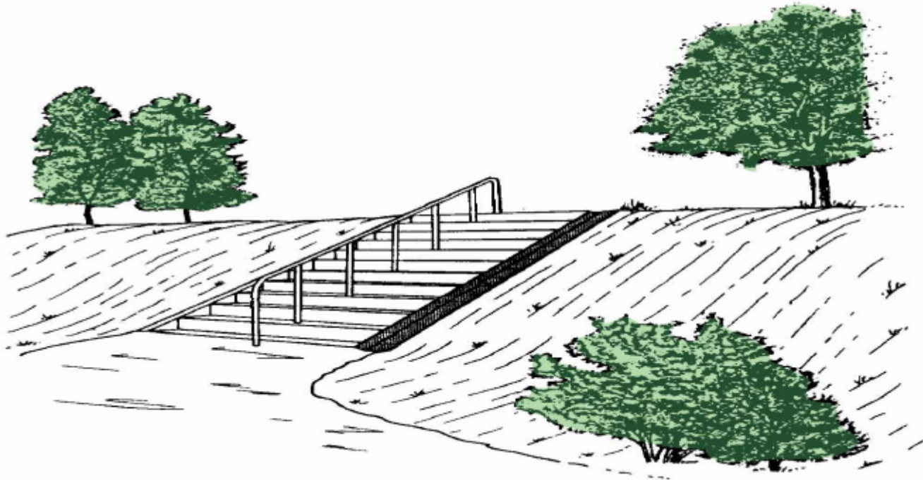
Stairs with a side ramp.
