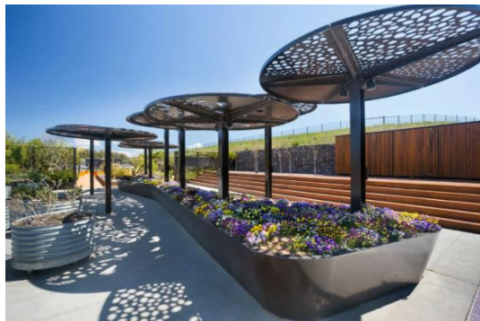
Example 2: Conceptual idea for Shade structures at Bus Stops and where shade is needed where trees are not able to be planted
