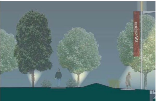
Decorative Lighting - Night view of tree uplights
