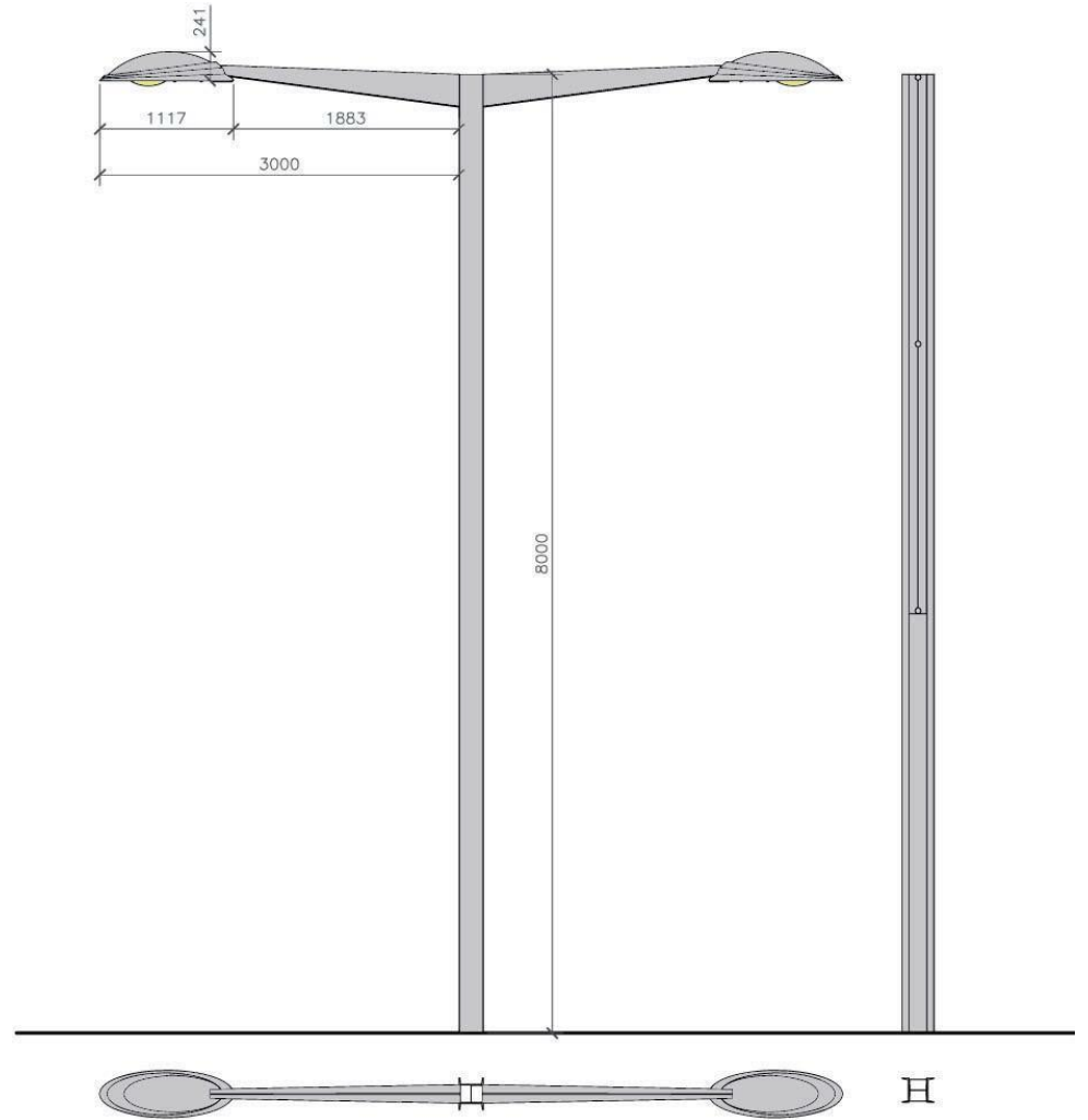
Centre median light standards to be used approaching the intersection of College and Huron Church
