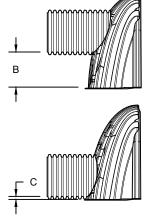
CUSTOM PARTIAL CUT INVERTS ARE AVAILABLE UPON REQUEST. INVENTORIED MANIFOLDS INCLUDE 12-24" (300-600 mm) SIZE ON SIZE AND 15-48" (375-1200 mm) ECCENTRIC MANIFOLDS. CUSTOM INVERT LOCATIONS ON THE MC-4500 END CAP CUT IN THE FIELD ARE NOT RECOMMENDED FOR PIPE SIZES GREATER THAN 10" (250 mm). THE INVERT LOCATION IN COLUMN 'B' ARE THE HIGHEST POSSIBLE FOR THE PIPE SIZE.
