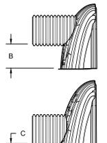
CUSTOM PARTIAL CUT INVERTS ARE AVAILABLE UPON REQUEST. INVENTORIED MANIFOLDS INCLUDE 12-24" (300-600 mm) SIZE ON SIZE AND 15-48" (375-1200 mm) ECCENTRIC MANIFOLDS. CUSTOM INVERT LOCATIONS ON THE MC-4500 END CAP CUT IN THE FIELD ARE NOT RECOMMENDED FOR PIPE SIZES GREATER THAN 10" (250 mm). THE INVERT LOCATION IN COLUMN 'B' ARE THE HIGHEST POSSIBLE FOR THE PIPE SIZE.
