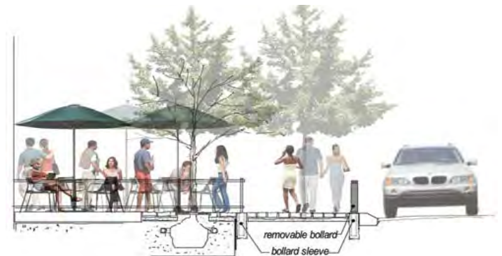
ABOVE: Rendering of a flexible sidewalk design for King Street in Kitchener, Ontario. Removable bollards are used to extend the sidewalk in the summer to maximize seating space for patios and make room for special events. In the colder months, the extra space can be used for more on-street parking.
