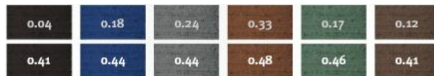
Figure 10: The albedo differences between standard (above) and cool coating (below) concrete tiles (Global Cool Cities Alliance, 2012)
