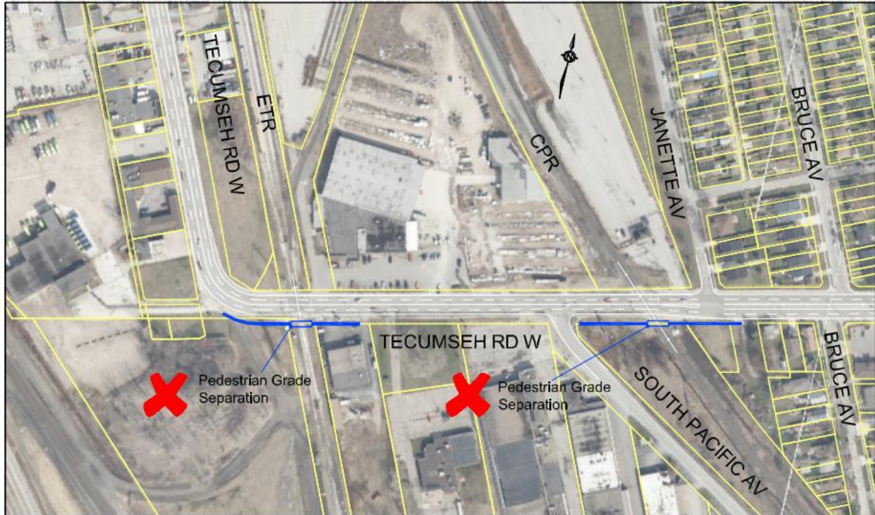
Figure 10: Cycling/Pedestrian Grade Separation
