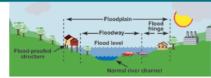
**Floodway:** The hazardous portion of the floodplain where flood depths and/or velocities are such that they pose a significant threat to life and/or property. The floodway is generally defined as the area required for the safe passage of flood flows.
