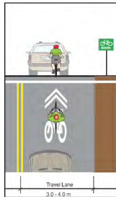
Cross-Sections of Shared Roadways – Narrow Signed Bicycle Route with optional sharrow (Source:OTM Book 18)
