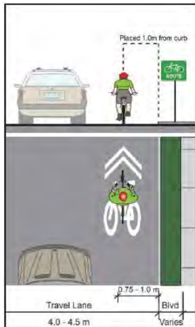
Cross-Sections of Shared Roadways – Wide Signed Bicycle Route with optional sharrow (Source:OTM Book 18)
