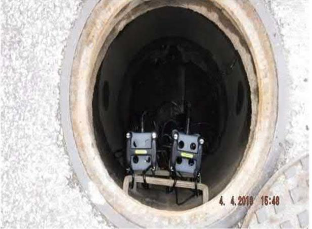
A view looking down into a manhole. Two electronic flow monitors are mounted on a wooden frame at the bottom of the manhole. The manhole is surrounded by concrete. A timestamp in the bottom right corner reads "4. 4. 2018 15:48".                         |
