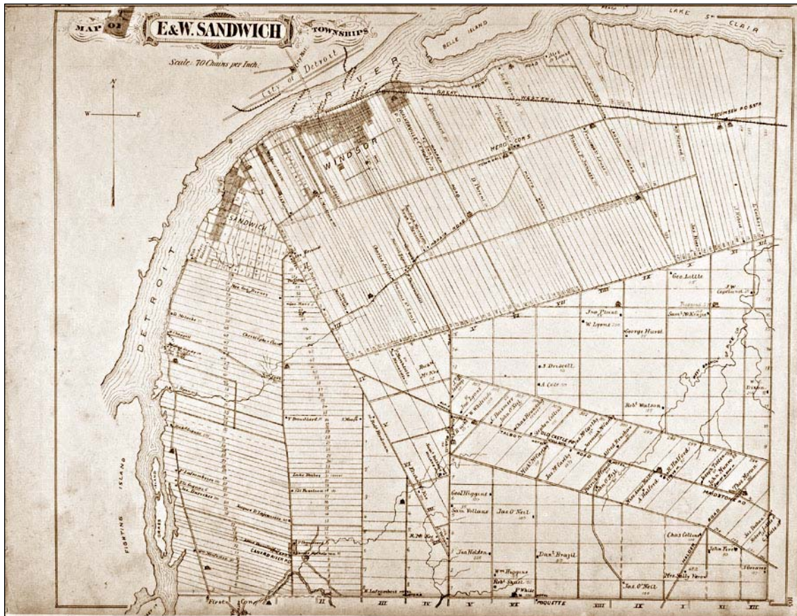
The East and West Sandwich Township map in the Illustrated Historical Atlas of the County of Essex (1881) shows the complex survey patterns of the former Township of Sandwich. Lauzon Road is noted as an open road allowance in Concessions 1, 2 and 3 in the northeast part of East Sandwich Township.
