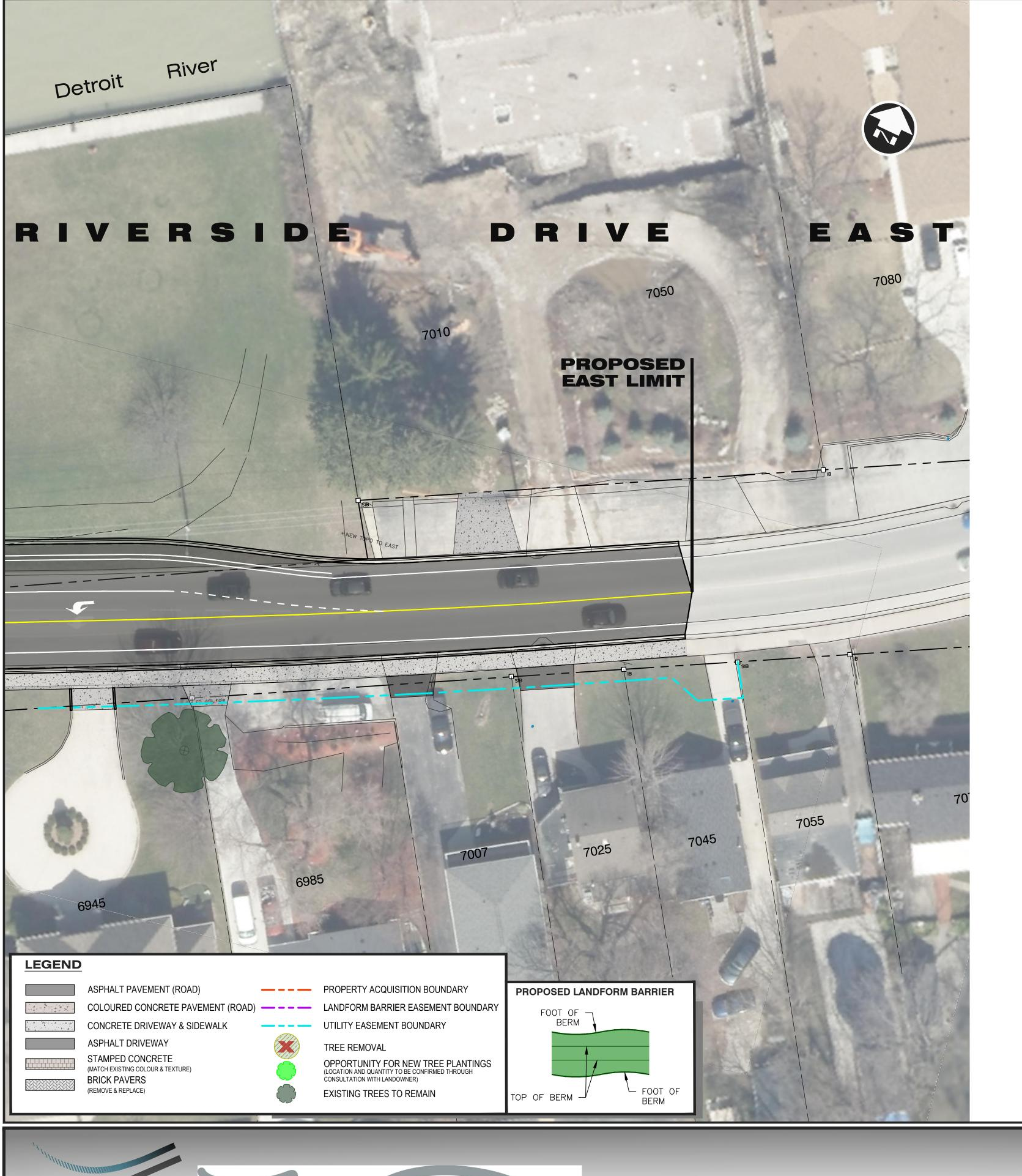
DETAILED LANDFORM BARRIER, LANDSCAPE, STREETLIGHT AND UTILITY DESIGN IS UNDERWAY AND ADDITIONAL TREE TRIMMING WILL BE REQUIRED TO ACCOMODATE LANDFORM BARRIER CONSTRUCTION AND INSTALLATION OF THE PROPOSED AERIAL POWER DISTRIBUTION LINE.
