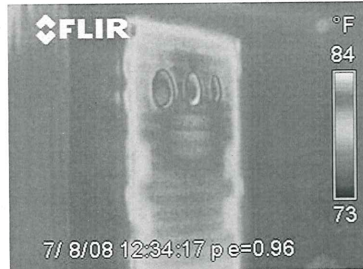
Infrared Picture reveals that it is indeed a hollow core door.
