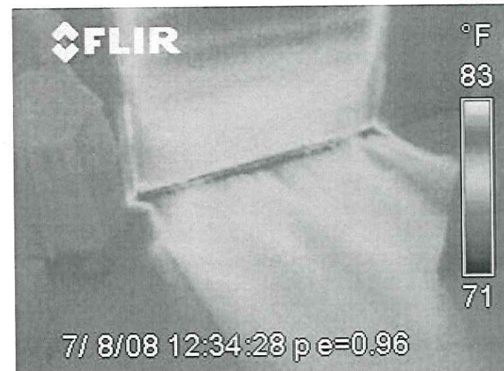
... air leaking at bottom weather stripping.
